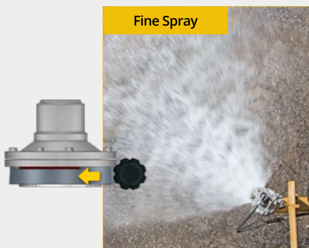
The “fine” spray head opening is 1/4 inch tall. This setting results in a finer spray of water with maximum reach and width at high pump speeds. This is the recommended setting for most water distribution applications.
